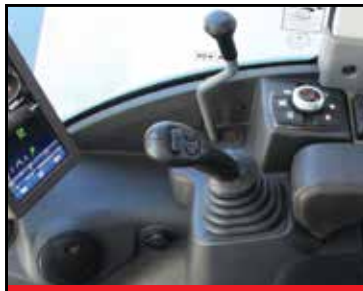
Hydraulic Pilot Controls
