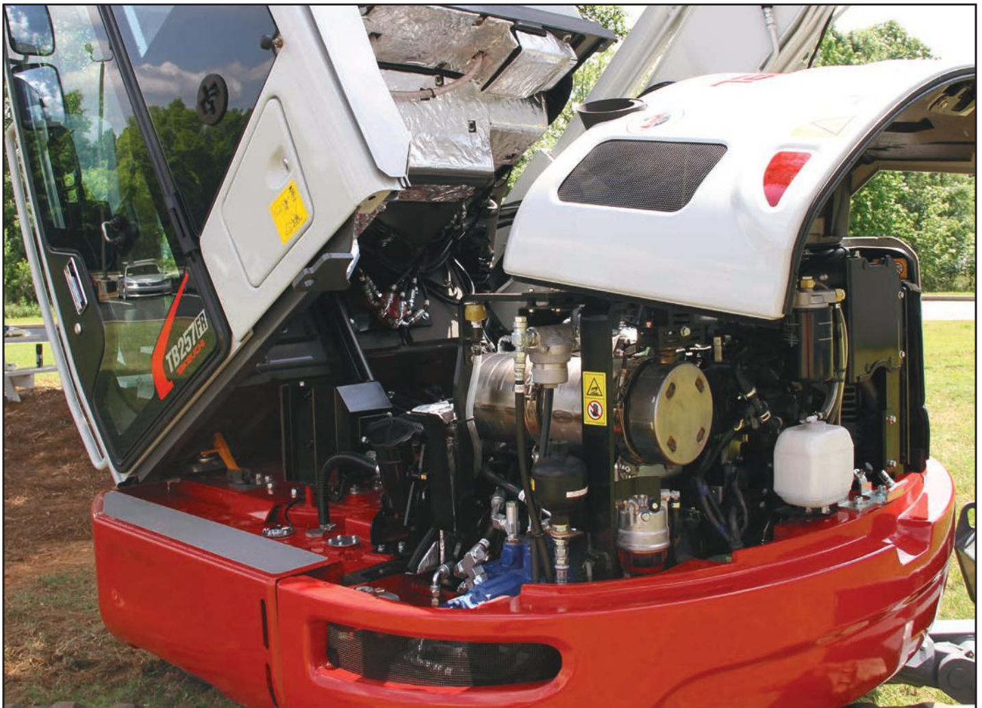
Forward Tilting Cabin and Wide Opening Service Hoods Provide Exceptional Maintenance Access.
