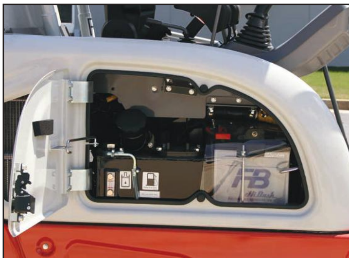
Lockable Service Door - Fuel Fill, Hydraulic Tank & Battery
