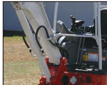
Main Boom Cylinder Guard
