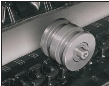
Triple Flange Track Rollers
