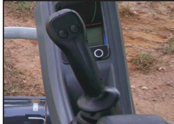
Pilot Operated Controls
