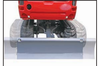
Retractable Track Frame
